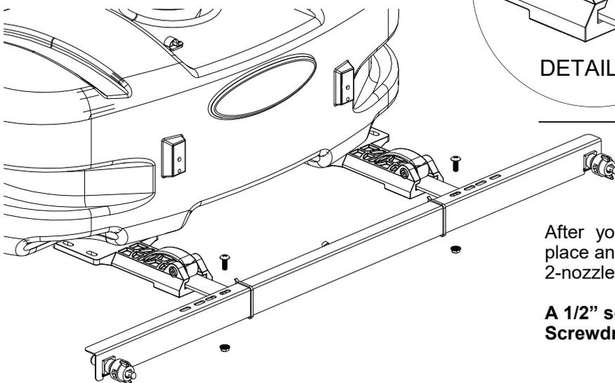
After your boom mounting brackets are secured in place and the unit secured on your ATV, attach the 2-nozzle boom in place with (2) screws and whiz nuts.
