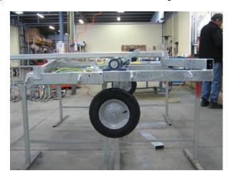
Lower the suspension and fit the wheels
