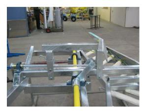
If required, bolt the tank bracket onto the spine making sure there is enough clearance for full travel of the suspension quadrants.
