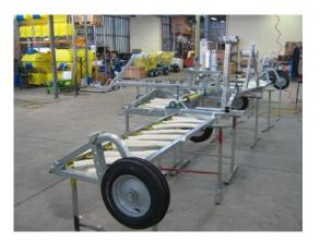
Fit the drawbar. Fit and plumb tank if required. Adjust the suspension, outer wheels and drawbar to suit the operation.
