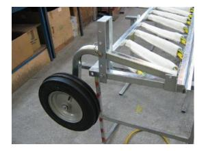
Fit the wings to the main frame – use washers as spacers on the shoulder bolts if required. Fit the RH & LH axles and height adjusters. Fit wheels to all the axles.
