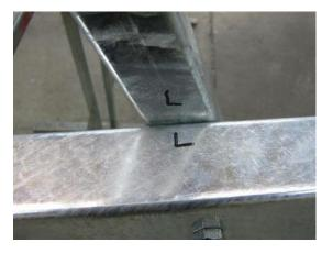
Bolt the "A" frames into position – note that the frames fit on the forward side of the rear crossmember. These are marked with "R" and "L" on both the "A" frame and the rear crossmember to aid assembly
