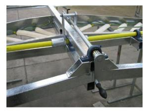
Bolt the pillow block bearing to the frame and bolt the "T" piece to the quadrants.
