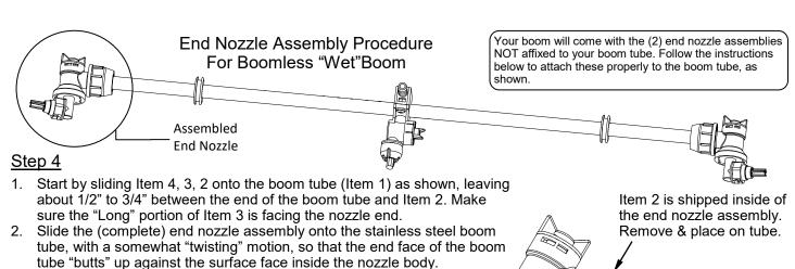
3. Now push the "compression olive" (Item 3) against O-ring (Item 2) and slide (both) into the nozzle body opening firmly.
