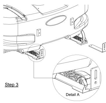
After your tank brackets are securely attached, turn the tank assembly over and position it so that the cam handles which extend beyond the back of the tank are facing you and just hanging over the edge of the table or flat surface you are assembling this on.
