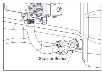
Checking/Cleaning the sprayer's filter/screen:
