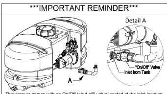
This sprayer comes with an On/Off (shut-off) valve located at the inlet location of the tank, towards the underside. (See Detail A). You must make sure the valve is in the "open" position before using your sprayer.
