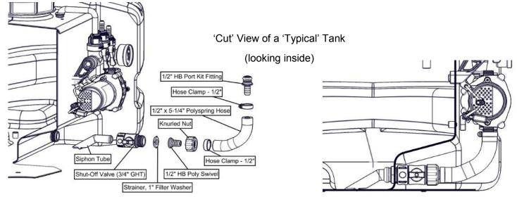
The suction line of your sprayer should contain a 'siphon tube' or intake tube which should be rotated so that it just touches the bottom of the tank surface. (see Detail Views). Reach in and rotate it, as needed, if not already in this position.
