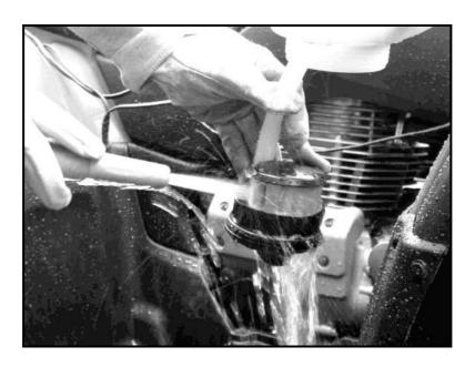
Each HGSR spray gun has a built-in filter in the spray tip. Unscrew the red spray tip holder from the lance nut to expose the tip filter. Pull the lance nut back to reveal the filter. Rinse under a hose and replace the filter element in the spray tip (the dished side faces toward the trigger).
