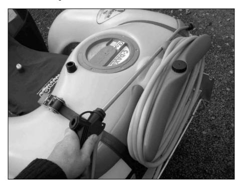
Connect the Sprayrider™ electrical connector (at front of the tank) to the battery cable.
