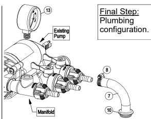
With your pump (Not Included) mounted on the 'top' of your tank this is how your bypass line will be configured. You may need to punch or drill the hole for your return line, approx. 7/8".
