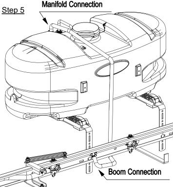
After your nozzle harness is attached to the boom, locate the 48" hose and the (2) hose clamps from the parts bag.
